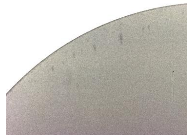
Fig.1 X-ray topo of Si wafer after thermal stress
