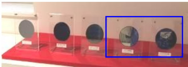
Fig.1 Display Si wafer (Left : before liftoff, Right : after liftoff )
