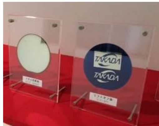
Fig.2 extended photo of lift off wafer
