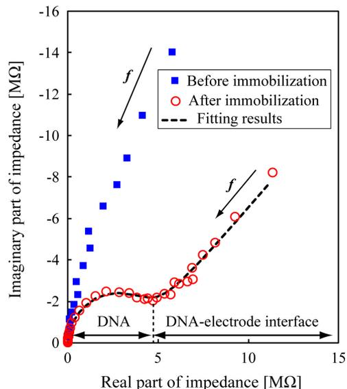
Fig. 1. Complex impedance plot between microelectrodes before and after DNA stretch/immobilization.
