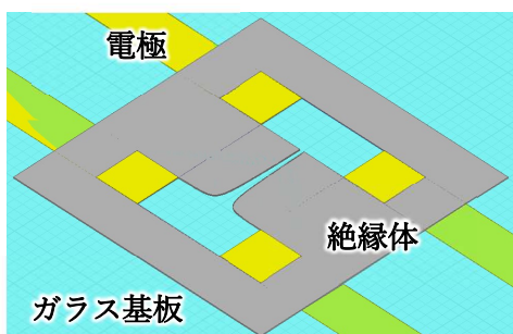
Fig. 1 Structure of Insulator-Based DEP Device
