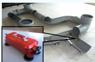
Pipe Inspection Robot
