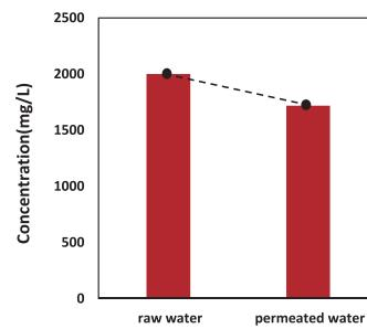
Figure 2: Concentration of Li<sup>+</sup> in raw water and permeated water
