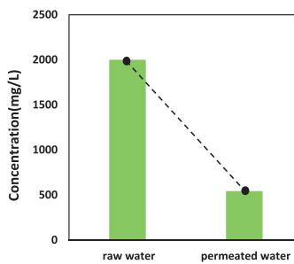
Figure 1: Concentration of Mg<sup>2+</sup> in raw water and permeated water
