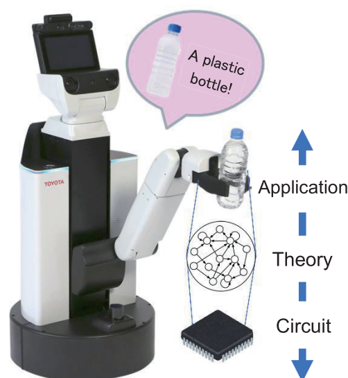
Fig. Example of Robot Object Recognition by Reservoir Chip
